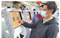
It Uses a 19" Infrared Non-Contact Touch Screen that Allows The User to Complete All Check-in Procedures by Hovering Their Fingers Over the Screen Instead of Touching it
